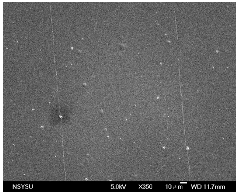
Figure 4.68 SEM surface morphology of the deformed ZrCu/Cu (25 nm/25 nm) multilayer sample at a high magnification of 350X.
