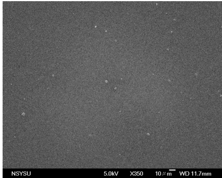
Figure 4.32 Surface morphology of the undeformed ZrCu/Cu (10 nm/10 nm) multilayer sample at a low magnification of 350X.
