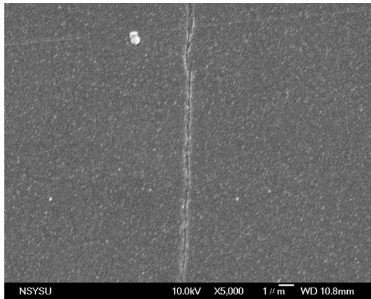
Figure 4.66 SEM surface morphology of the deformed ZrCu/Cu (50 nm/50 nm) multilayer sample at a high magnification of 5000X.
