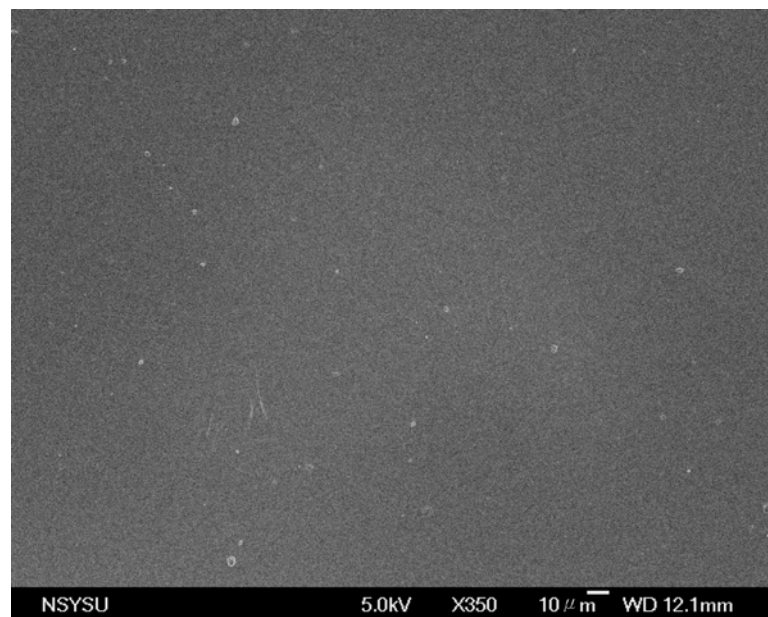
Figure 4.21 Surface morphology of the undeformed ZrCu/Cu (50 nm/50 nm) multilayer sample at a low magnification of 350X.
