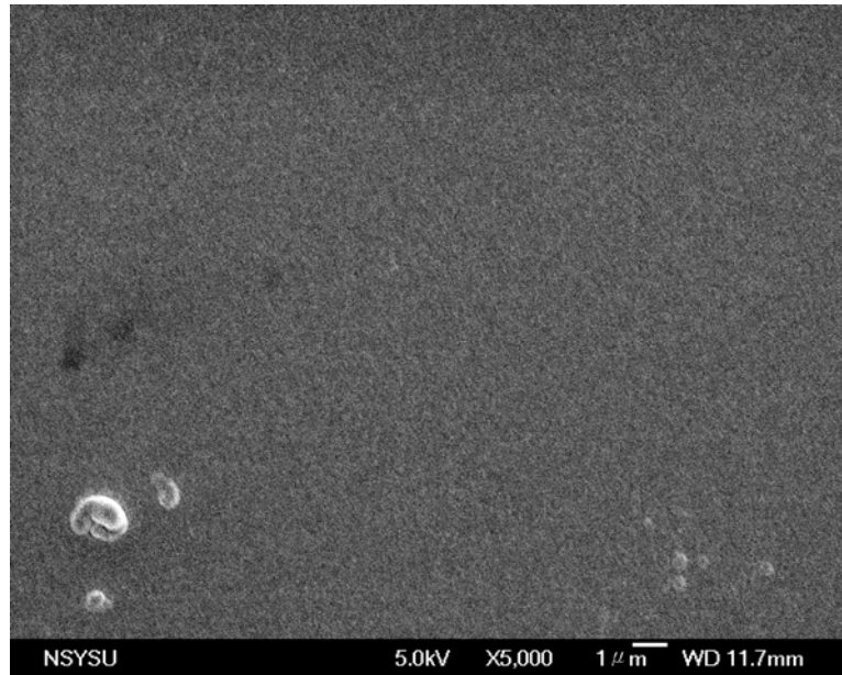
Figure 4.34 Surface morphology of the undeformed ZrCu/Cu (10 nm/10 nm) multilayer sample at a high magnification of 5000X.
