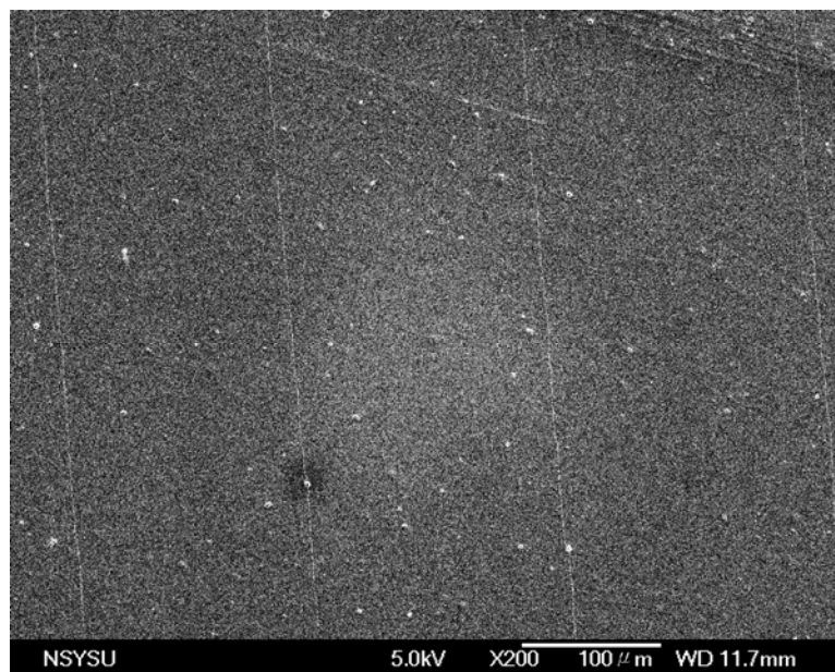
Figure 4.67 SEM surface morphology of the deformed ZrCu/Cu (25 nm/25 nm) multilayer sample at a high magnification of 200X.
